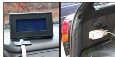
Left: A mileage counting device mounted to the dashboard. Right: A transmission device located in the rear of the vehicle reports the mileage at refueling.
